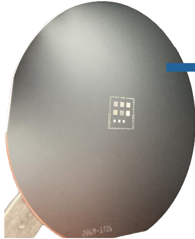
Single-die freeform master made by 2GL
