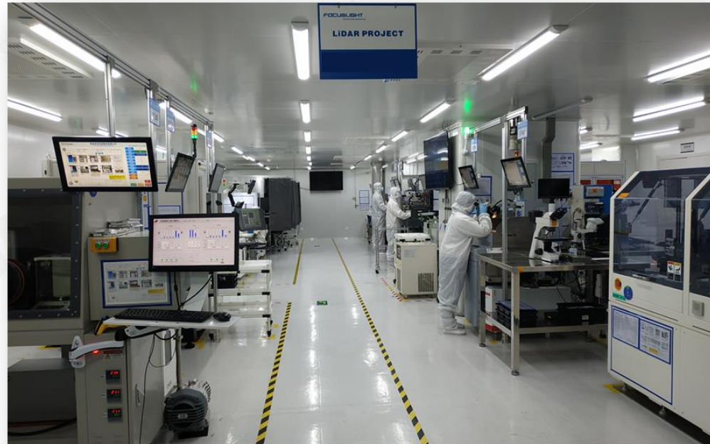
Mass production line of 3D flash LiDAR laser module in Focuslight
