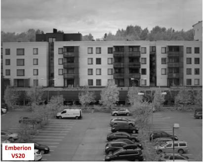
The non-linear response characteristic and the wider spectral sensitivity range of Emberion cQD sensor offer a wider dynamic range, see the contrast differences in the clouds, balconies and car windows.
