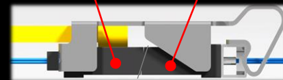
MT ferrule attached to CSOP lid MT ferrule part of fiber cable to be plugged in
