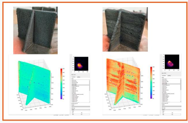
3D part thermal gradient reconstruction using information provided by CLAMIR\* Left: the part is built using CLAMIR laser power control Right: the part is built with constant laser power and NO control
