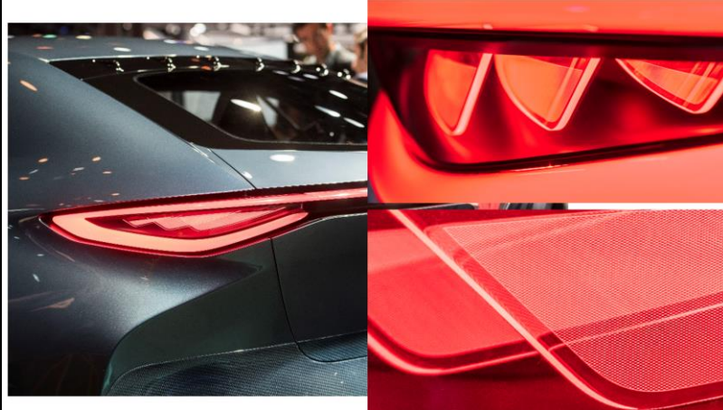
Micro-optics on PMMA prototype parts
