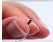
1.35mm outer diameter flexible scope
