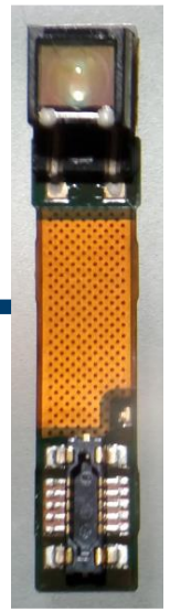
Integrated 3D Sensing Module (NIR CCM, RGB CCM, LPM)
