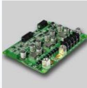
High power laser diode drivers
