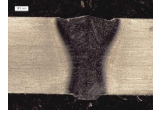
Ti-6Al-4V; 3.2mm; butt joint; Ar shield gas
