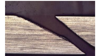
Fan shaped hole; Inconel 718 (TBC). Film cooling holes increase efficiency of cooling air by 30%, reducing the amount of air required for cooling.
