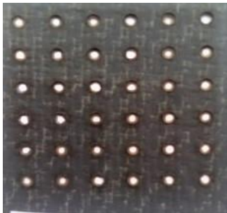
Carbon Fiber Pre- Preg, the amount of burn back on the top surface is only a few tens of microns
