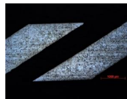
Uncoated 2.2mm thick Hastelloy-X; 30 degree from surface; hole dia. 0.50-0.75mm
