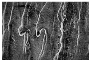
2mm thick Al-Li alloy reinforced with 20% (wt.) SiC particulate; QCW laser; N 2 assist gas
