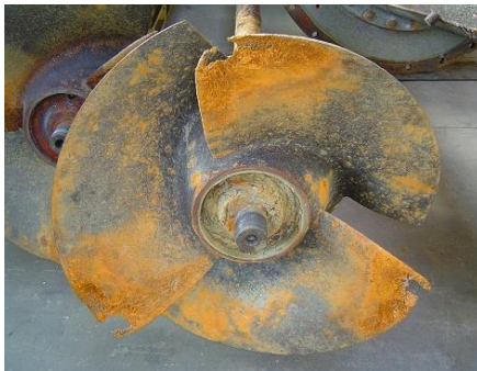
Cavitation on water pump propeller
