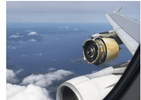
Damaged engine of Airbus A380, Credit: Jacob Soboroff (Twitter @jacobsoboroff) 2017
