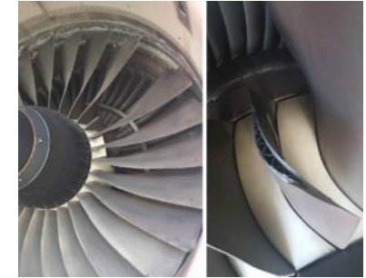
Fractured blade of AirAsia engine failure. Credit: avherald.com 2020
