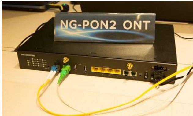
ONT: Optical Network Terminal
