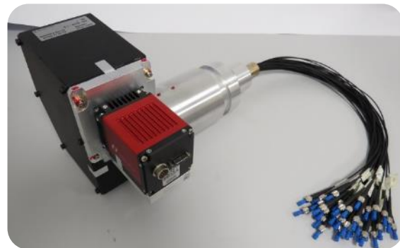
NIR Multichannels (38 channels) spectrometer
