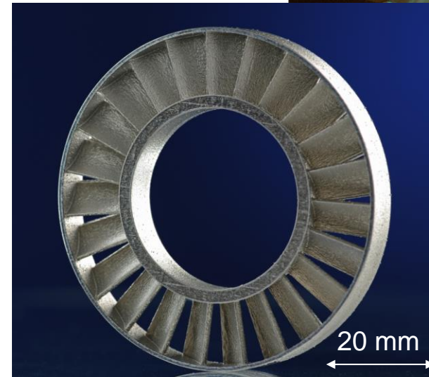
TiAl part printed via LBM
