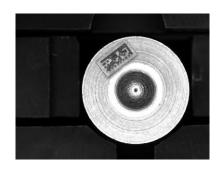
b) identify component angular position detect laser/mechanical marking
