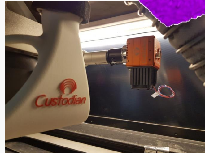
TACHYON 16k CAMERA PLUS coaxially integrated in a PBF machine
