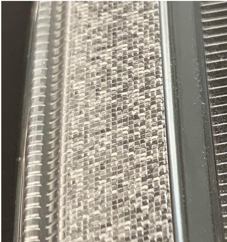
Texture engraved directly over PMMA part (prototype)
