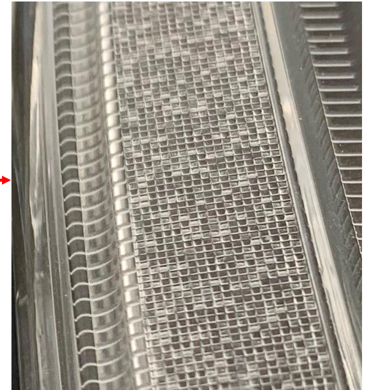
PMMA part injected in texturized mold (production)
