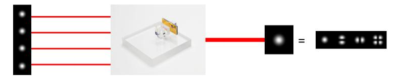
→ Efficient beam combiner with optimal beam quality
