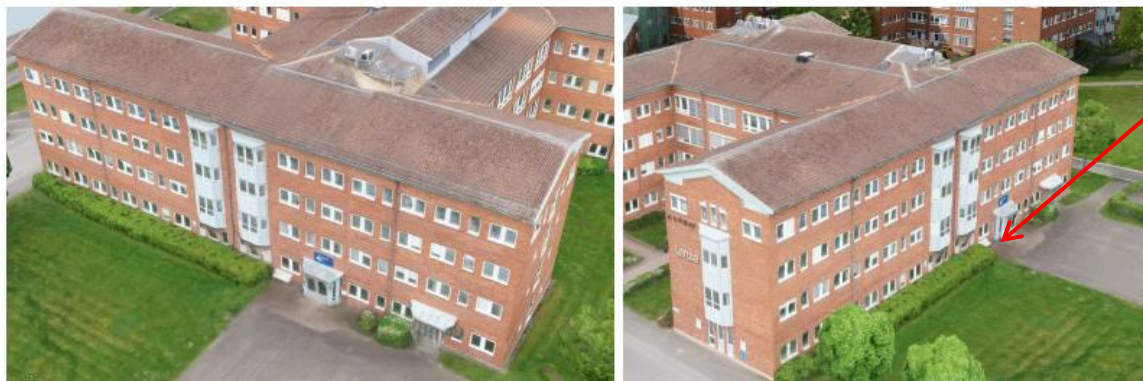
(b) Two views of the resulting 3D model created by Spotscale AB, in these pictures shown with texture from an "ordinary" RGB camera.
