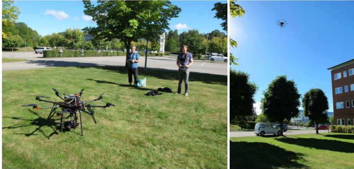
(a) Acquiring image data by flying in circuits around an office building.
