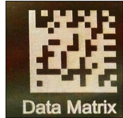
Material: Stainless Steel Pulse Width: 200 ns Repetition Rate: 200 kHz
