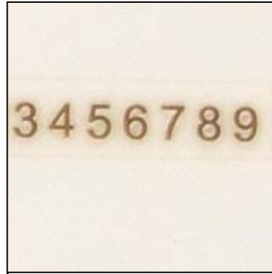
Material: Alumina Pulse Width: 200 ns Repetition Rate: 36 kHz, x10
