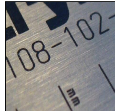
Material: Stainless Steel Pulse Width: 10 ns Repetition Rate: 500 kHz
