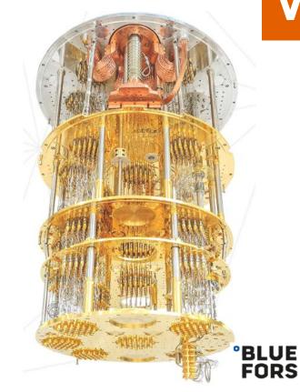
The state-of-the-art cryostat (Bluefors Oy) with control RF cabling (220 coaxial cables).
