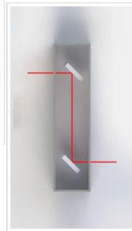
Lateral Transfer Hollow Retroreflector & Periscope (LTHR & LTHP)
