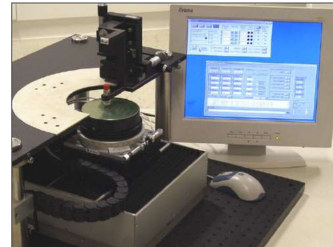
An early - 2002 - 2" wafer VCSEL tester
