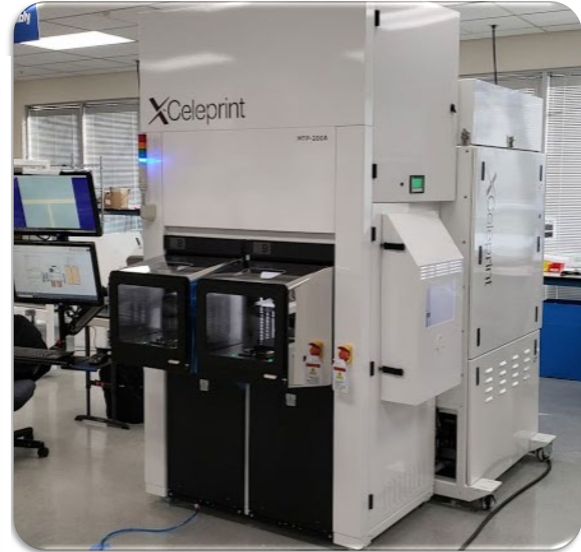
Transfer-printer with automated substrate handling
