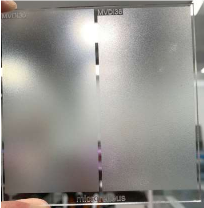
VDI30 and VDI 36 engraved directly over PMMA
