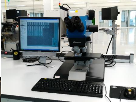
Passive bare die inspection
