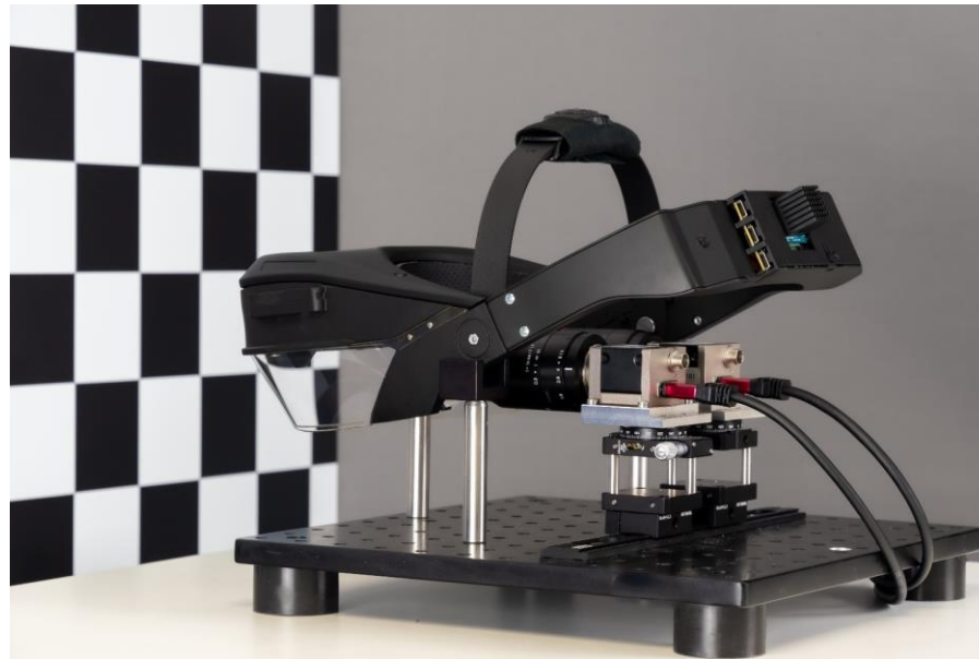
Distortion measurement for AR-glasses
