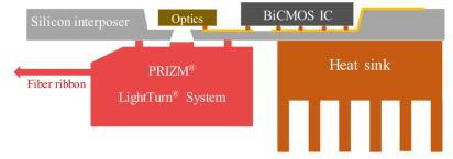
12-Channel 10 Gb/s Optical Transmitter and Receiver
