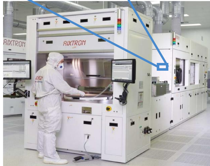
deposition system (e.g. MOCVD)
