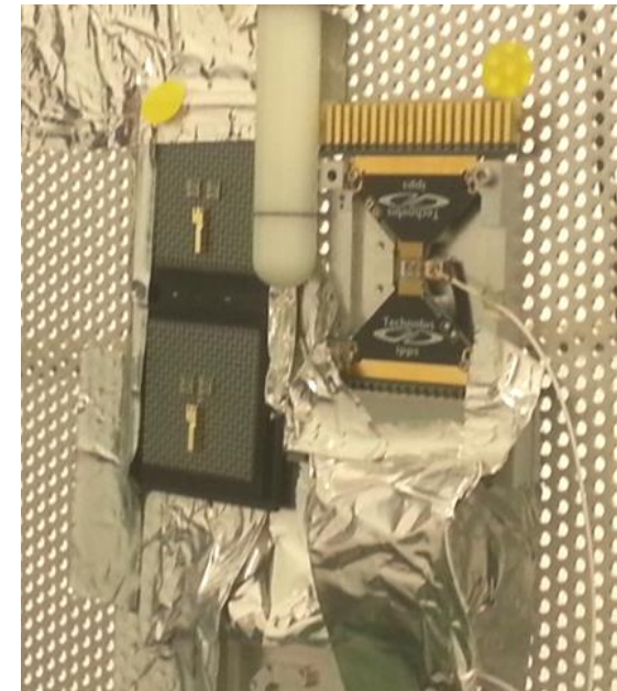
ESTEC test facility Co-60: alignment of dies and package for live-monitoring during irradiation
