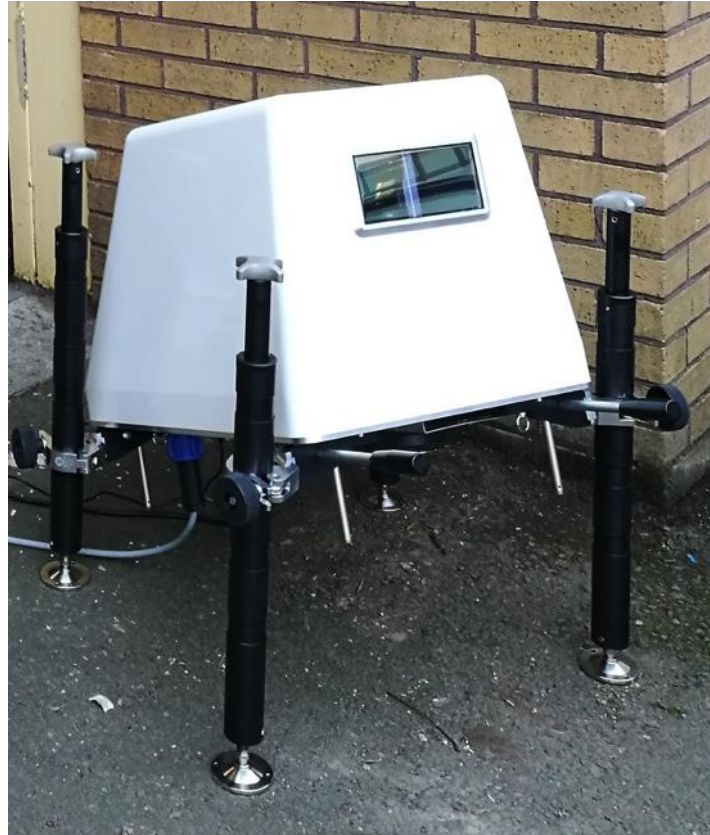
Low-cost Doppler wind LIDAR prototype produced by Fraunhofer CAP. The beam is emitted through a fixed window, reducing system complexity and lowering the unit cost.
