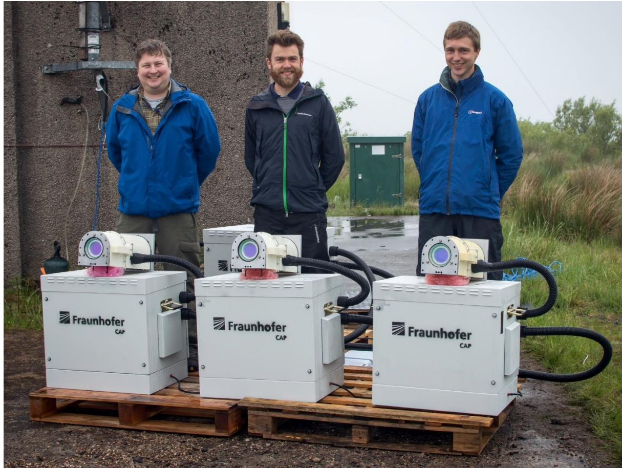
Multi-beam coherent Doppler wind LIDAR prototype being tested by making comparison measurements with a calibrated met-mast
