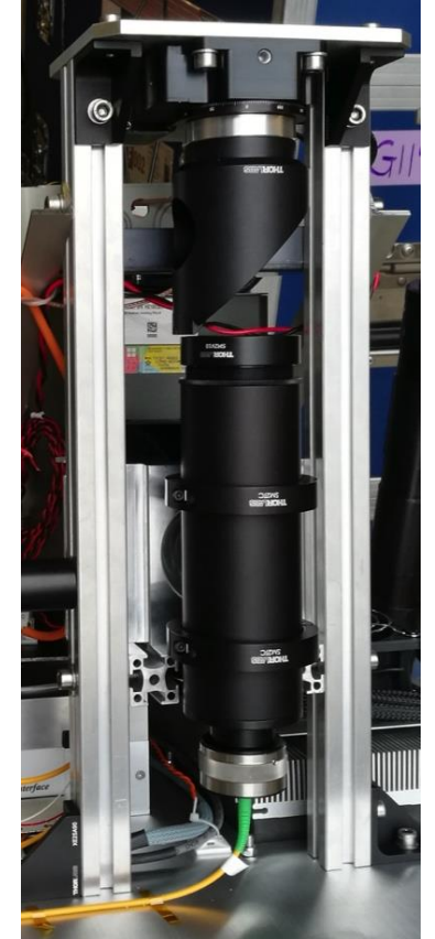
Rugged Risley prism beam scanning module developed in house and motion compensated platform under test at Fraunhofer IPA, Stuttgart
