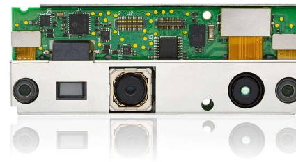
Integrated 3D Sensing Module (NIR CCM, RGB CCM, LPM)
